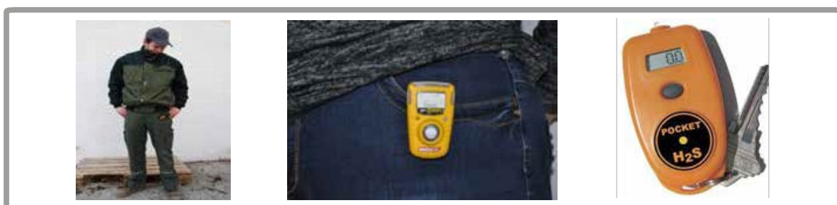
The photos above show various types of gas detectors. These detectors can be carried in various ways. They may be fastened to clothes, placed on a key ring, held in the hand, or worn on a lanyard around the neck.
